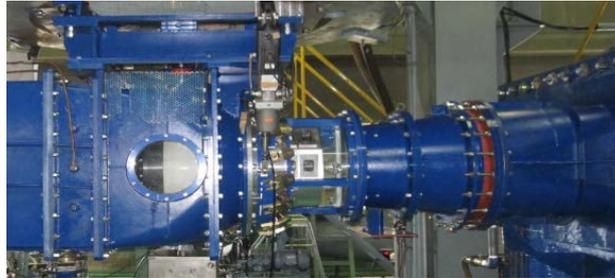
**Figure 3.** Model test equipment for Model hydro turbine
