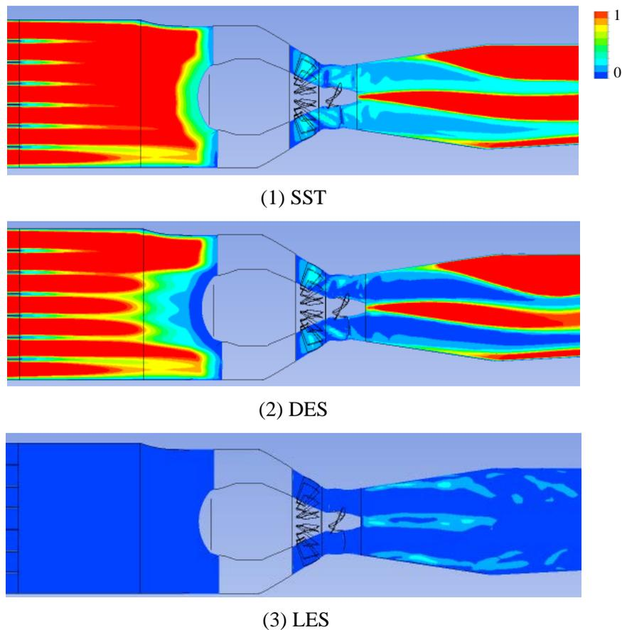
**Figure 12.** Eddy viscosity contour
