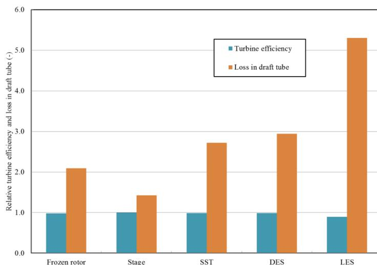
**Figure 6.** The comparison of efficiency and draft tube loss between the numerical and experimental results
