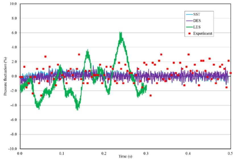
**Figure 11.** Runner outlet pressure fluctuation comparison between experimental and numerical results
