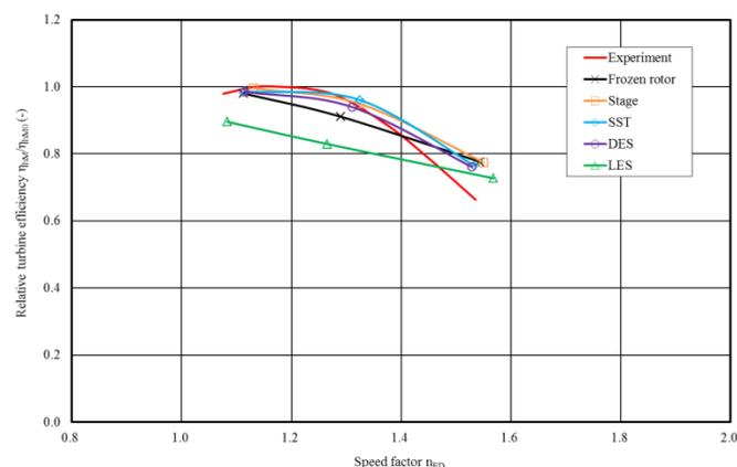
**Figure 4.** The comparison of efficiency between the numerical and experimental results
