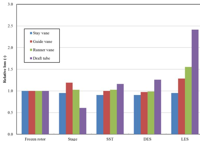
**Figure 5.** The comparison of hydraulic loss between the numerical and experimental results
