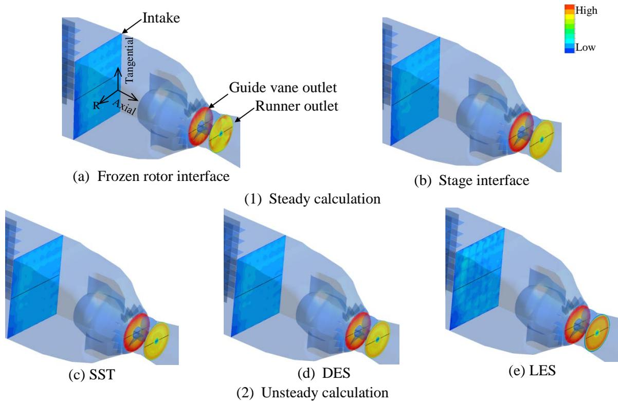
**Figure 7.** Flow velocity distributions at intake, guide vane outlet and runner outlet
