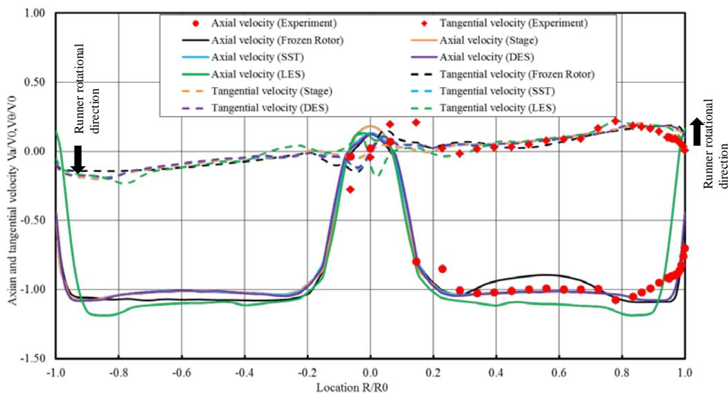
**Figure 10.** Flow velocity distributions numerically simulated and experimentally measured at runner outlet
