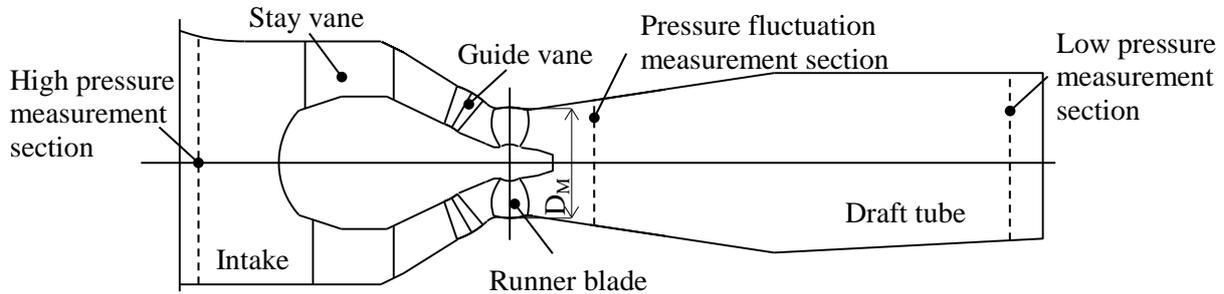
**Figure 1.** Configuration of  $N_{QE}$  0.8 Bulb model turbine
