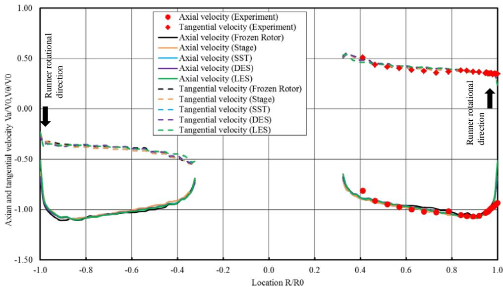
**Figure 9.** Flow velocity distributions numerically simulated and experimentally measured at guide vane outlet
