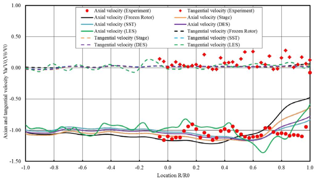
**Figure 8.** Flow velocity distributions numerically simulated and experimentally measured at intake
