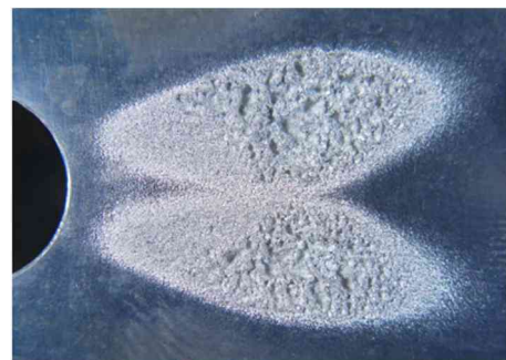
Fig.3 Cavitation Erosion after 100 hour Exposure
