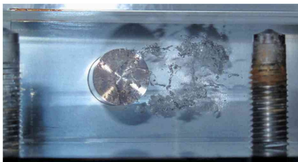
Fig.2 Cavitation at the downstream of the pin
