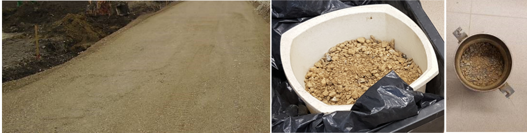
Figure 2. Views of the construction layer built from recycled aggregate and the sample of recycled aggregate
