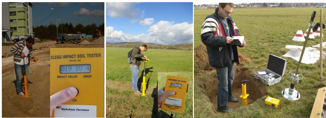
Figure 6. Testing the degree of compaction of earth plane by Clegg Impact Soil Tester with indicating the CIV reading
