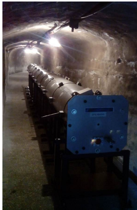
Figure 1. Shock tube in underground experimental base of the Mining Institute
