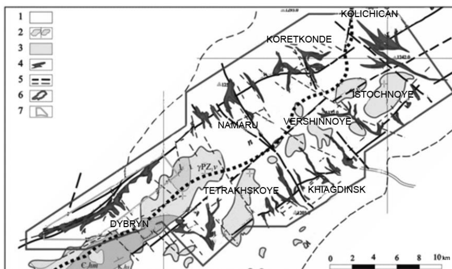
Figure 1. Overview geologic map of Khiagdinsk ore field (according to the data presented by JSC “Rusburmash”): 1 – Neogene deposits; 2 - 3 basement rocks: sedimentary (a) and metamorphic (b) (2), granitoids (3); 4 – uranium-ore deposits; 5 – discontinuous faults of different types; 6 – the contour of Khiagdinsk ore field.
