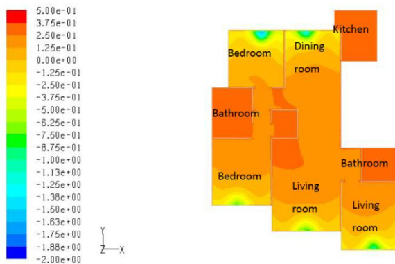
Figure 8. PMV distribution of wall type ventilator with heat exchange
