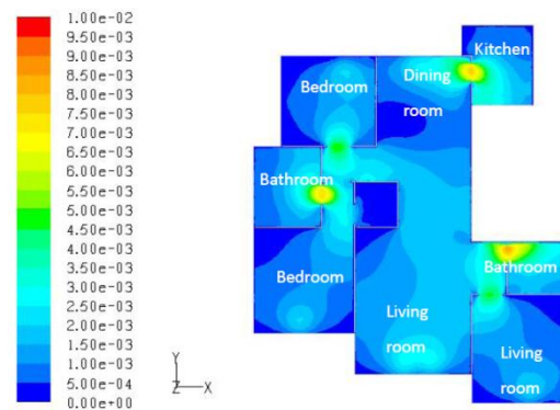
Figure 3. Air velocity field of natural inlet and mechanical exhaust
