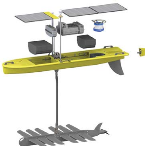
Figure 1. 3-Dimensional layout of the Wave Glider.
