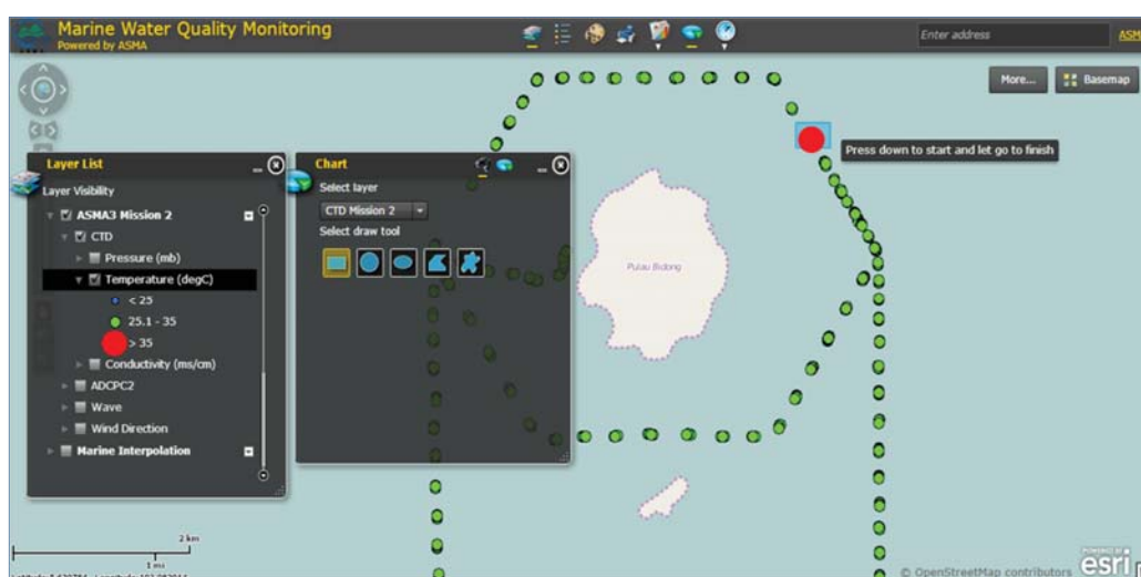
Figure 8. Colour coded ranges and instantaneous colour schemes for each monitoring locations.
