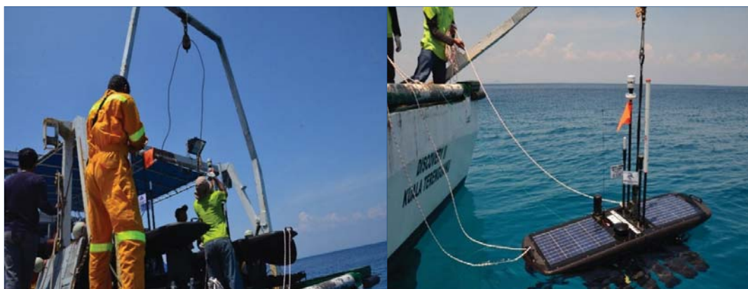
Figure 3. On-boat preparation before the launch of the Wave Glider. Figure 4. The Wave Glider is ready for launch and begin mission.
