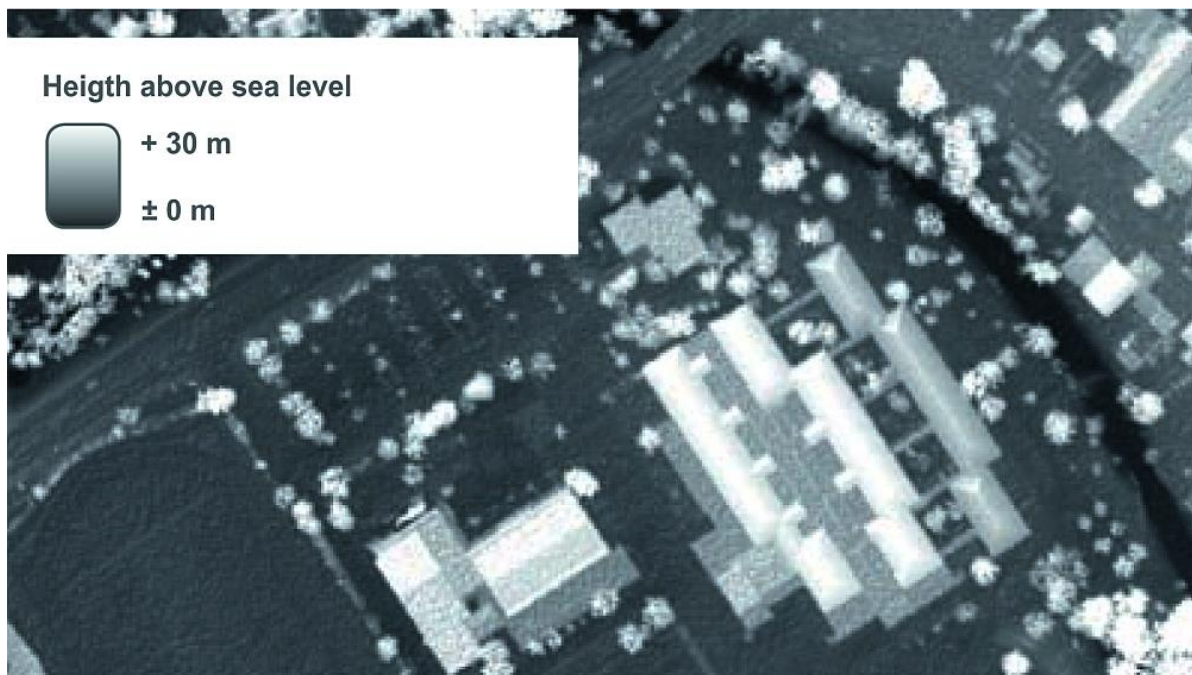
Figure 1. The Digital Object Model made of airborne laser scan data
