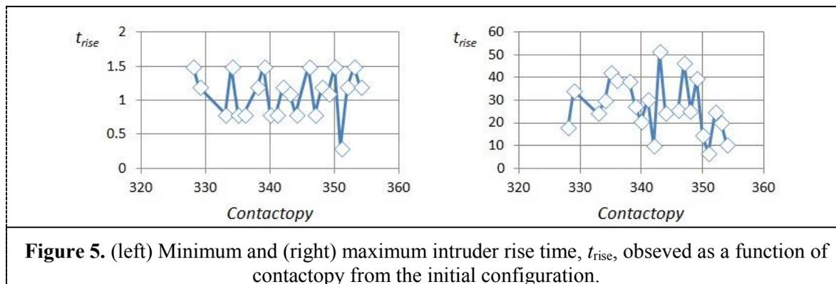
**Figure 5.** (left) Minimum and (right) maximum intruder rise time,  $t_{rise}$ , observed as a function of contactopy from the initial configuration.
