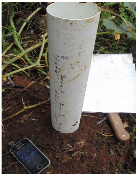
Figure 1. Simple Single Infiltrometer Device
