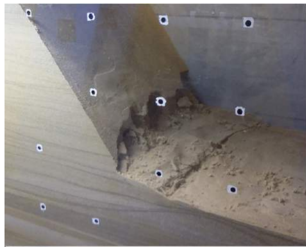
Figure 7. Local failure at the slope toe after 1800 hours of rainfall ( I = 87.7\text{mm/hr} ).
