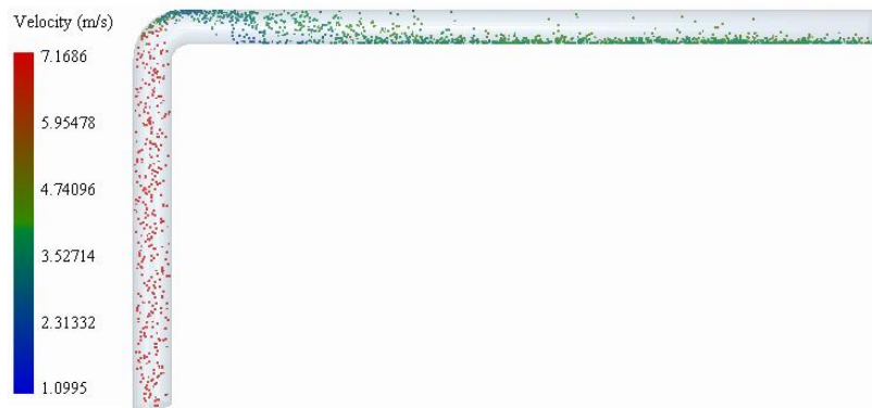
Figure 4. The solid flow structure and the particle velocity of vertical-horizontal case at t=2 s.
