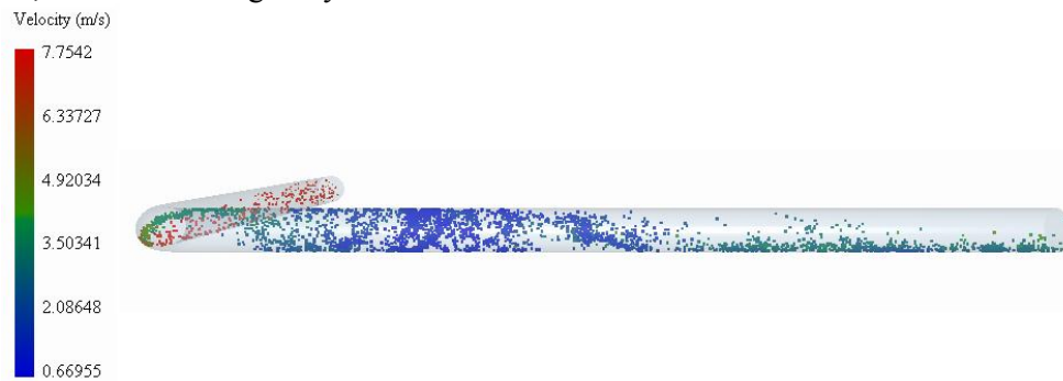
Figure 6. The solid flow structure and the particle velocity of horizontal-horizontal case at t=2s .
