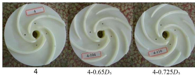
Figure 7. Test impellers of the three schemes.
