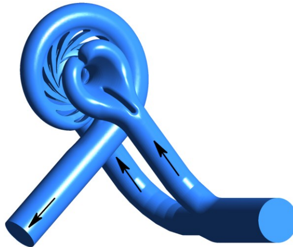
Figure 1. Computational domain of the pump. Arrows show flow direction.
