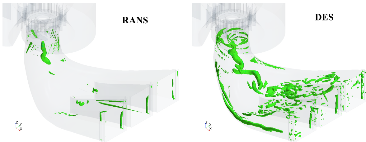
Figure 4. Isosurfaces of Q-criteria in the draft tube show the qualitative differences arising from the RANS and DES schemes for turbulence modeling
