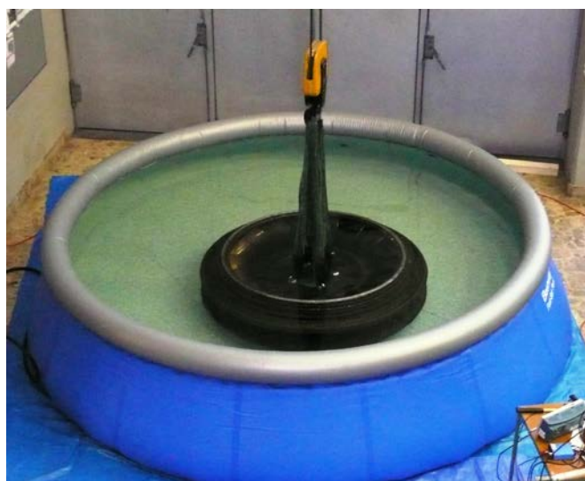
Figure 2. Experimental modal analysis in water
