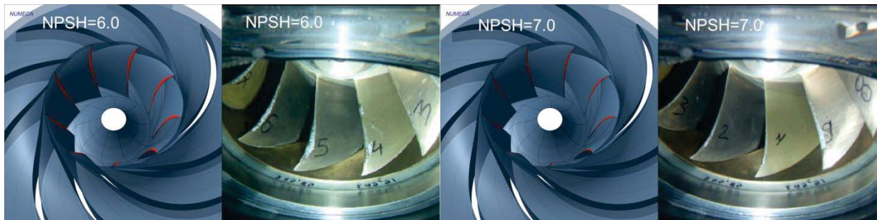
Figure 13. Comparison between numerical and experimental cavitation forms
