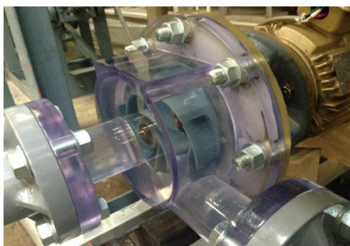
Fig.16 Visualization section of vortex pump
