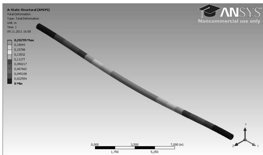
Figure 5. Deformations of a pipeline caused by ground settlement.
