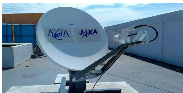
Figure 4. Outdoor unit; VSAT for Sentinel Asia Step2 in National Space Centre, Banting, Selangor
