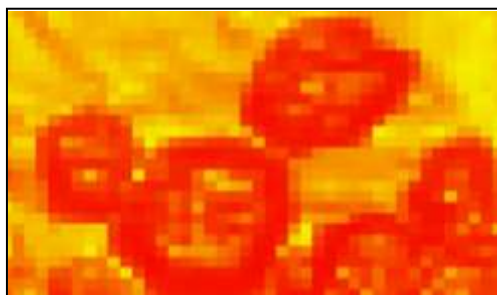
Figure 6a. Slope raster illustrates the steeper slopes that shaded red were determined as trees.
