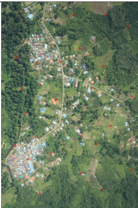
Figure 1. An example of aerial image with selected control points.
