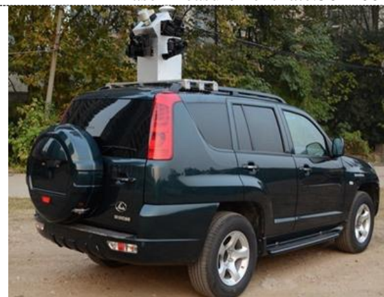
Figure 5. SSW Vehicle-borne laser scanning system
