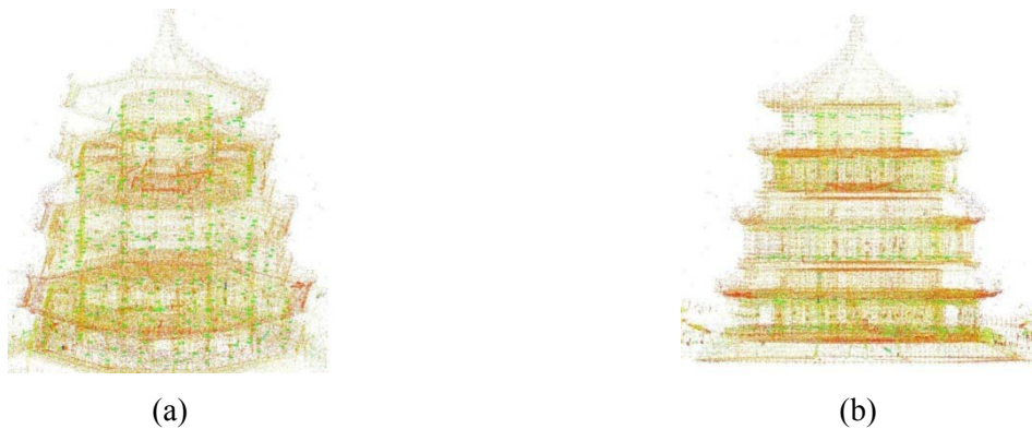
Figure 5. point clouds of cross-sections of the pillars in the whole tower (marked as green in the above figures). Figure (a) is the oblique view from above where the pillars are seen more clearly; Figure (b) is the view from the front where the cross-sections can be seen more clearly)
