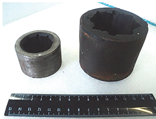
Figure 5. Rubberized sliding bearings of a water lift pump.
