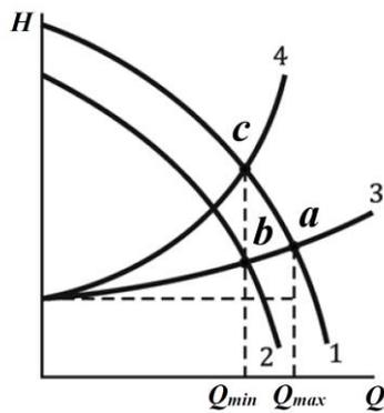
**Figure 4.** Static characteristics at nominal (1) and low (2) angular wheel speed pump, as well as when open (3) and partially closed (4) pipeline valves.
