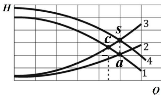
**Figure 2.** Effect of magnification hydraulic resistance network to choose pressure head pump characteristics.
