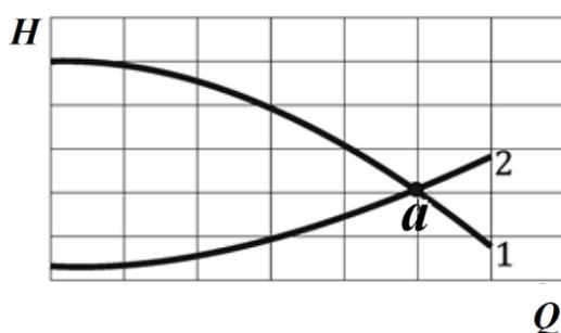
**Figure 1.** Pressure head pump characteristic and characteristic hydraulic network.
