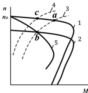
**Figure 5.** Mechanical asynchronous characteristics electric drive (1 natural, 2 - at frequency or cascade regulation, 5 Areostatnom regulation) and pumping unit (3 - with fully open, 4 – partially closed valve).
