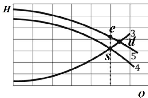
**Figure 3.** Influence of discrete power range on pressure head pump characteristic.
