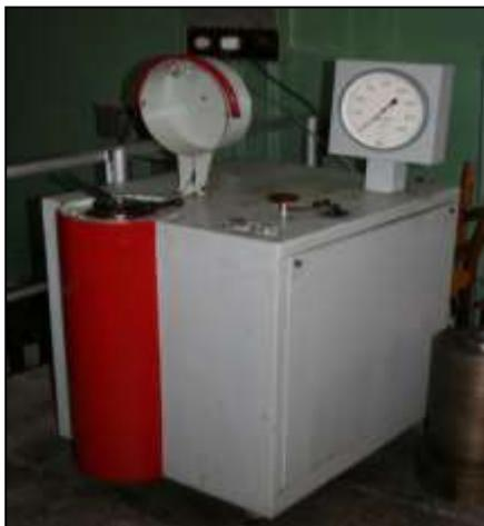
**Figure 1.** Experimental hydrostat for processing food products by ultrahigh pressure.
