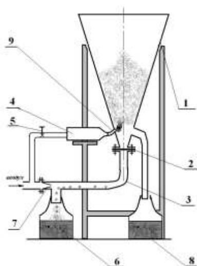
**Figure 2.** A device for the microencapsulation of ascorbic acid.
