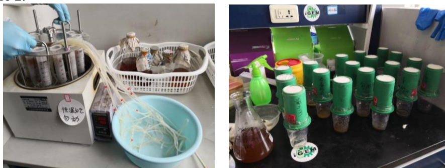
Figure 2. Tests of sand solidification with the perfusion method
