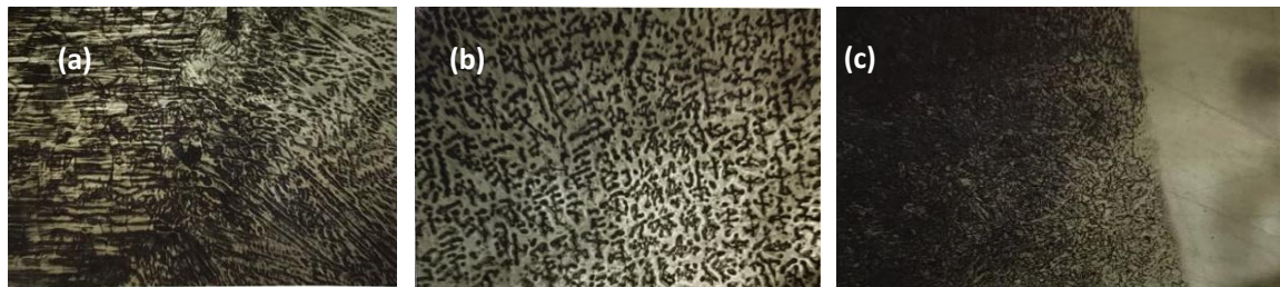
Figure 3. Microstructure of A-TIG welding joint. (a) HAV structure of 321 sides of stainless steel (b) Microstructure of weld (c) HAV structure of Q245R side of carbon steel.
