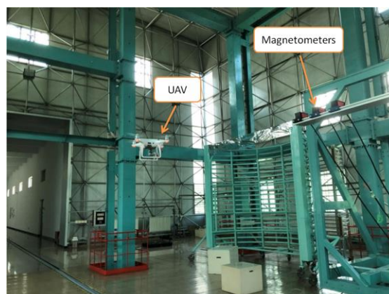
Fig. 5. UAV hover state position (1.2m far from the fluxgate magnetometers)
