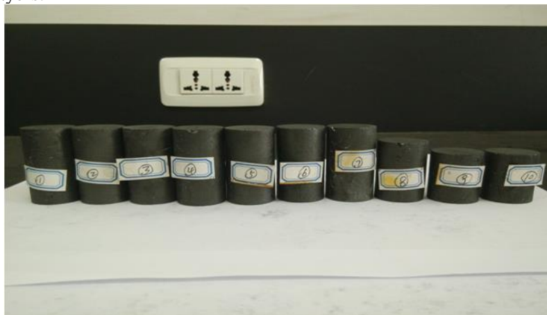
Figure 1. Core (cylinder) drilled from coal seam in block A of Xinjiang
