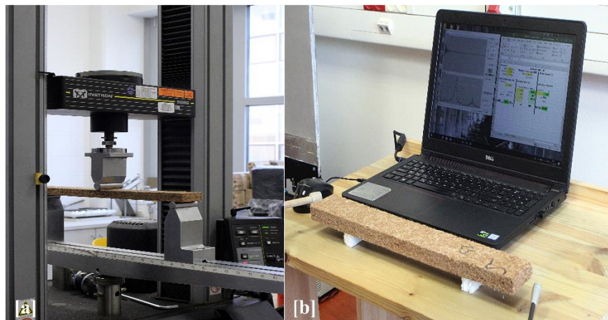
Figure 1 Determination of MOE through the destructive [a] and non-destructive tests [b]
