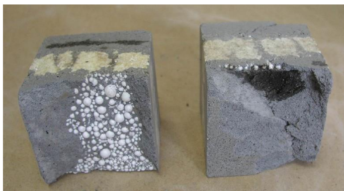
Figure 1. Destruction of Two- and Three-Layer Samples of Polystyrene Aerated Concrete
