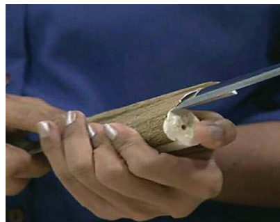
Figure 2. Slicing sesbania wood by manual method.
