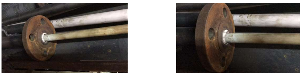
Figure 1. Physical diagram of damaged thermocouple
