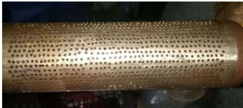
Figure 5. Disassembly diagram of the warm water filter in the low-pressure shaft seal.
