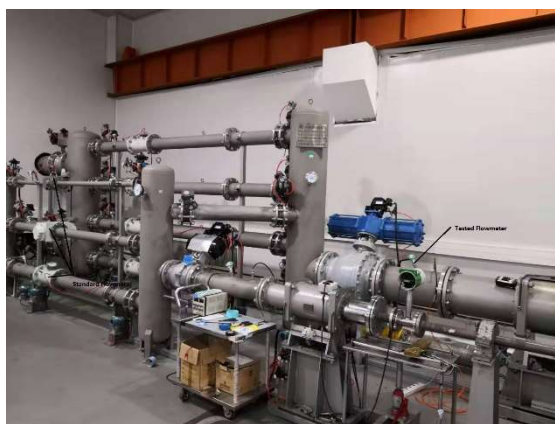
Figure 1. The gas flow standard device of standard meter method.
