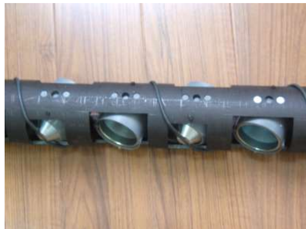
Figure 3. Adjustable jet angle perforator frame structure.
