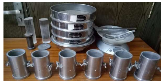
Fig.2 The main test tools and cylindrical crack specimen molds
