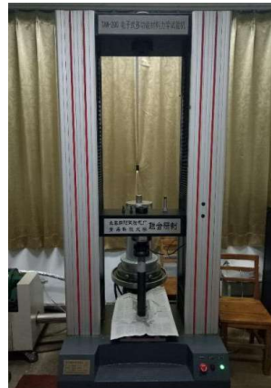
Fig.3 TAW-200 electronic multi-function material mechanics testing machine
