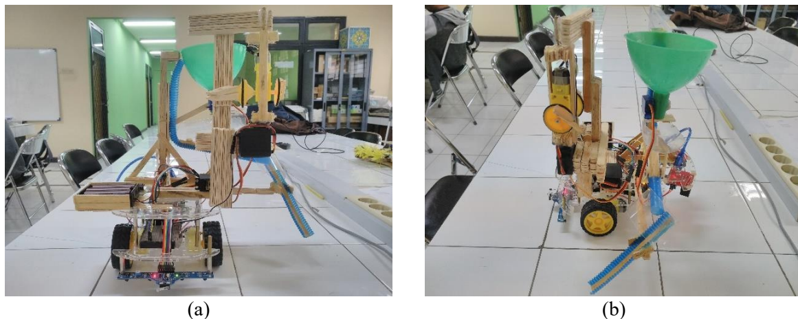
Figure 4. Implementation of the Seed-Planter Wheeled Robot (a) front-view, (b) side-view.
