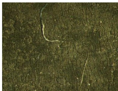
Figure 6. Surface of natural rubber based EBB pad after exposed to ozone
