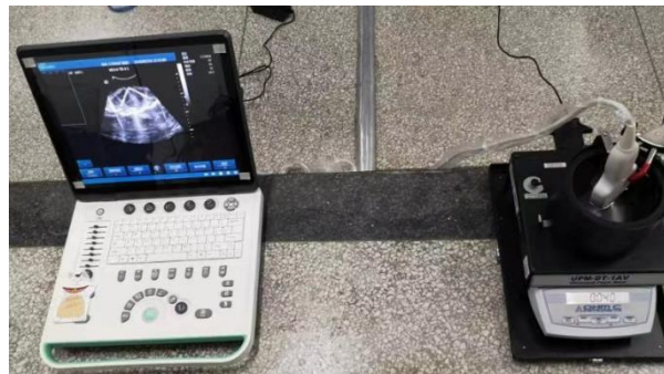
Fig.5 Measurement of Sound Field by Ultrasonic Power Meter
