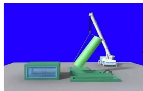
(b) Large diameter pipe installation simulation
