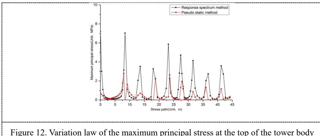
Figure 12. Variation law of the maximum principal stress at the top of the tower body
