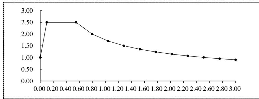
Figure 5. Designed response spectrum used in the calculation
