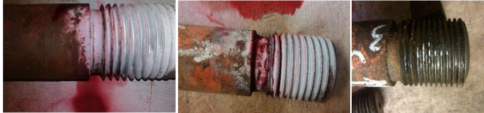
Figure 6. Penetration detection of hold-down bolts with cover setting ring.
