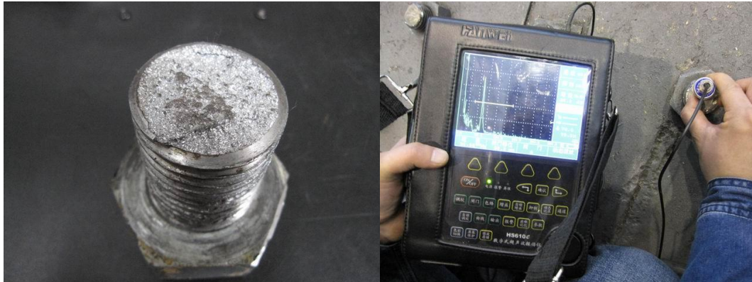
Figure 3. The tension bolt of rotor magnetic yoke is broken.
