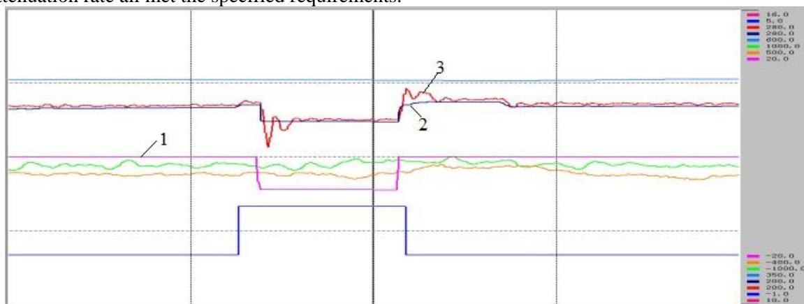
Figure 6. PFC disturbance test curve before transformation
