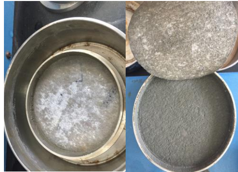
Figure 5. The anti clogging filter fabric after the test
