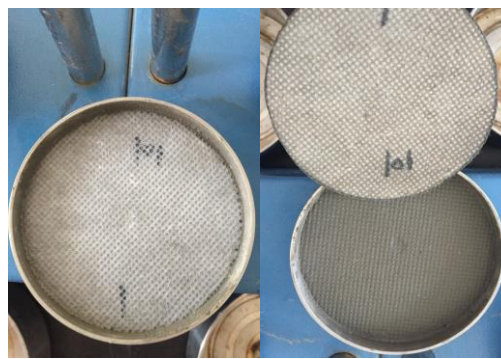
Figure 6. The anti clogging filter fabric after the test
