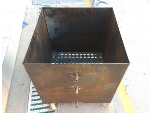
Fig 2. Structure simulation device of permeable parking lot
