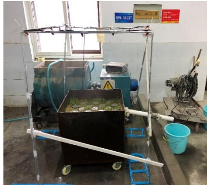
Fig 1. Artificial rainfall simulator
