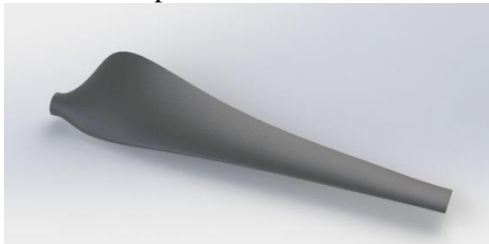
Fig. 5-1 3D solid model of NACA4412 airfoil
