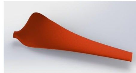
Fig. 5-2 3D solid model of NACA0009 airfoil
