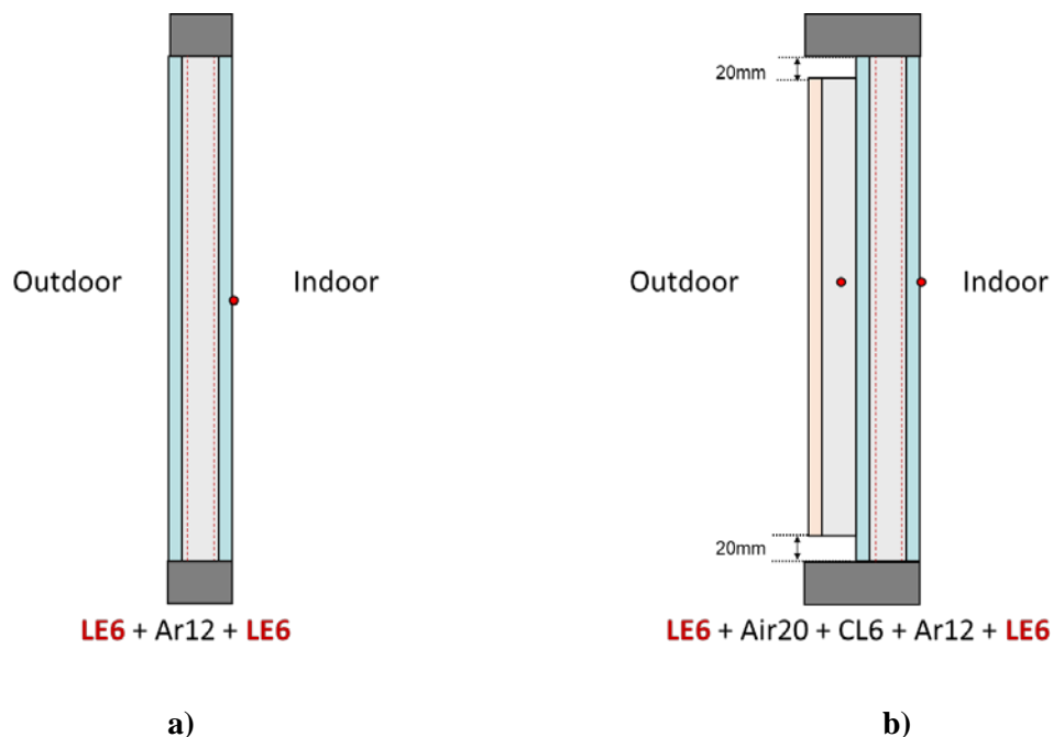
Figure 2 Schematic diagram widows and measurement points a) double glass, and b) SDSF
